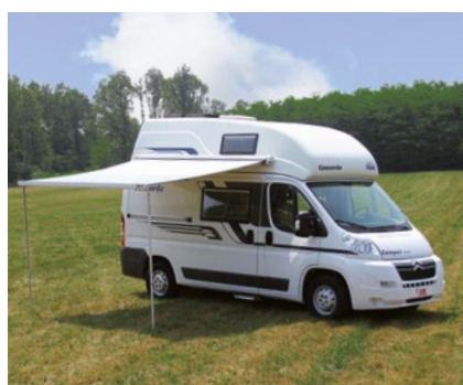
F45s: wall installation awning with specific brackets for Ducato vehicles
